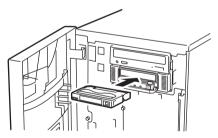
By fully inserting the data cartridge, it is automatically set in the drive and the TAPE MOTION LED lights.
